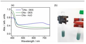
**Figure 4.** (a) Absorption spectra of  $^{NCN}CN_x$  in DES - 0.38 M TEOA solution (green trace) and aqueous 0.38 M TEOA (black trace) prior to irradiation with simulated solar light.  $^{NCN}CN_x^*$  absorption spectra in DES-0.38 M TEOA solution (blue) recorded in ambient air. (b) Photo of  $^{NCN}CN_x^*$  in DES solutions exposed to air (left) and in inert atmosphere (right).
