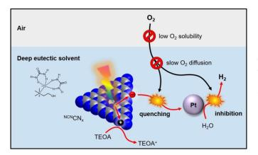
**Figure 1.** Schematic representation of solvent-mediated oxygen-tolerant photocatalytic hydrogen production in deep eutectic solvents demonstrated in this work.
