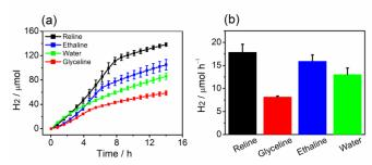
Figure 2. Photocatalytic  $H_2$  generation in DESs at  $Pt/^{NCN}CN_x$ : (a)  $H_2$  production in different DESs and water; (b) max.  $H_2$  production rate in DESs vs.  $H_2O$ . Conditions:  $^{NCN}CN_x$  (2.0 mg),  $H_2PtCl_6$  (0.05 mg Pt), in 2 mL DES (12.5% v/v  $H_2O$ , 0.38 M TEOA, 2 mM MV<sup>2+</sup>) or water (0.38 M TEOA, pH 7, no MV<sup>2+</sup>); AM 1.5G, 1 sun,  $40^{\circ}C$ , constant  $N_2$  purge.
