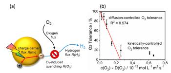
**Figure 6.** Mechanistic model for the solvent-induced  $O_2$  tolerance. (a) Schematic illustration of fluxes to and from the photocatalyst particle. (b) Plot of the  $O_2$  tolerance for  $H_2$  evolution versus the product of  $D(O_2)$  and  $c(O_2)$  in the respective reaction medium fitted according to eqn. 3.
